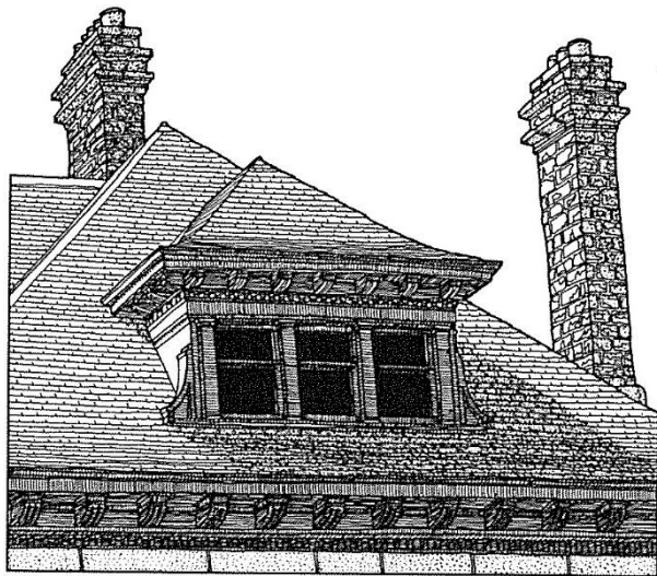
Figures 11, 12 Hip dormer [drawing by Paul B. Ohannesian. Image used with the permission of Touch Wood Editions] and wall dormer. Prominent roof slopes with skillful use of dormers to create living space within the roof form. Exquisite masonry chimneys further enhance the roof design.
